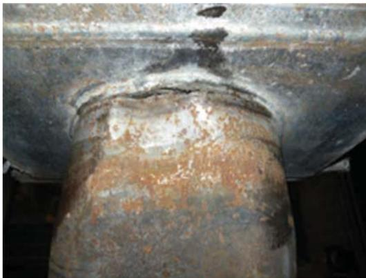
**Fig. 16.** Crack in Specimen B7 in the outside tube at the specimen to foundation beam connection**Table 8.** Cross-Section Deformations of Specimen B5
