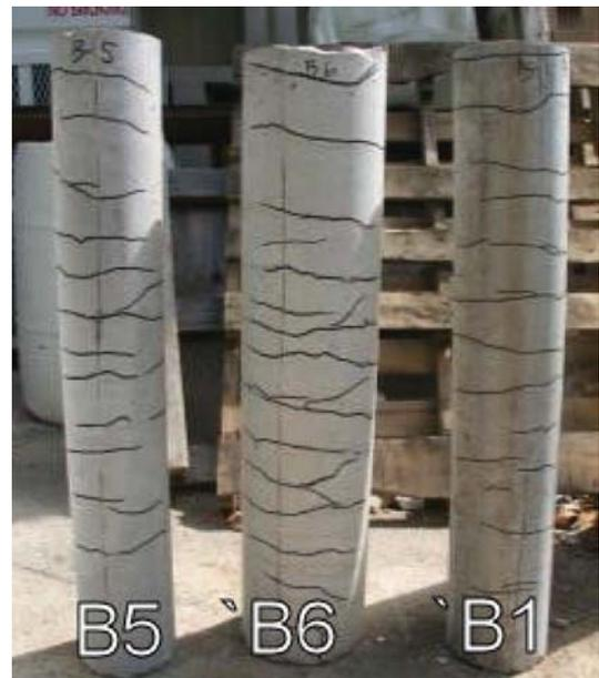
**Fig. 23.** Crack pattern in the upper part of Specimens B5, B6, and B1
