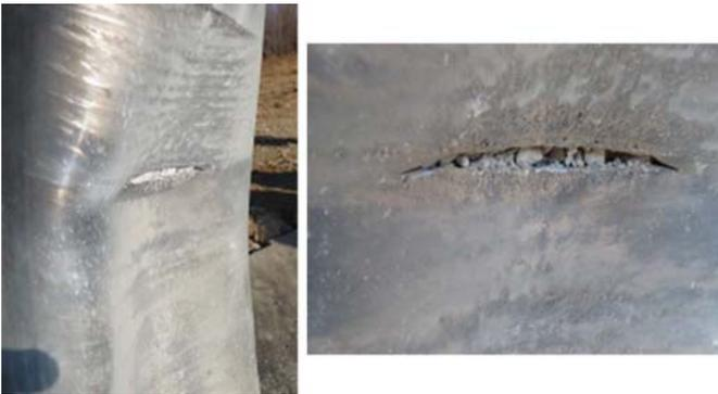
**Fig. 15.** Crack in Specimen B7
