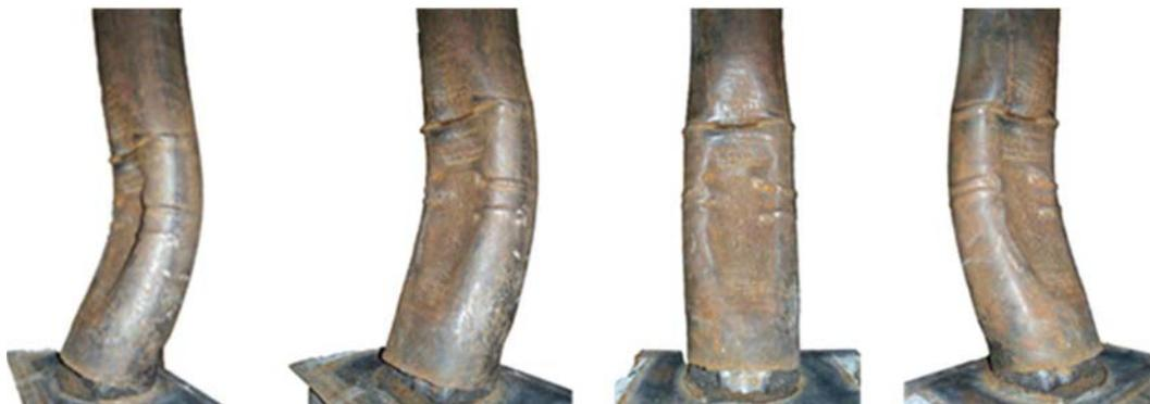
Fig. 20. Denting and fracture of Specimen B6
