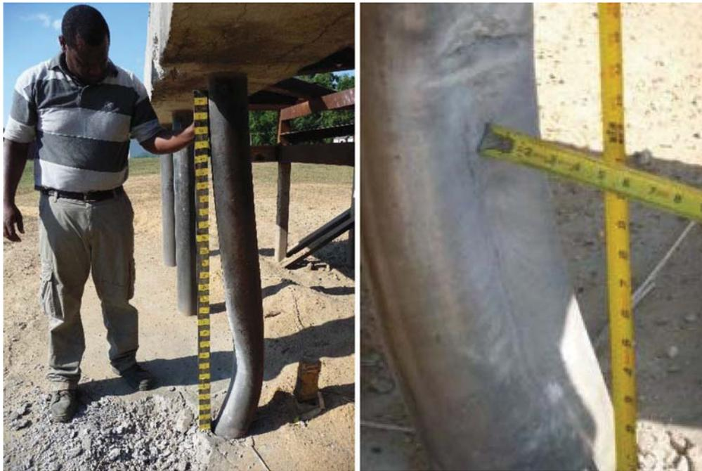
**Fig. 21.** Observed deformation of Specimen B9 (images by P. Fouché)
