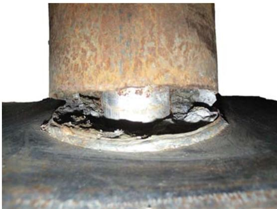
Fig. 19. Fracture at the base of Specimen B2
