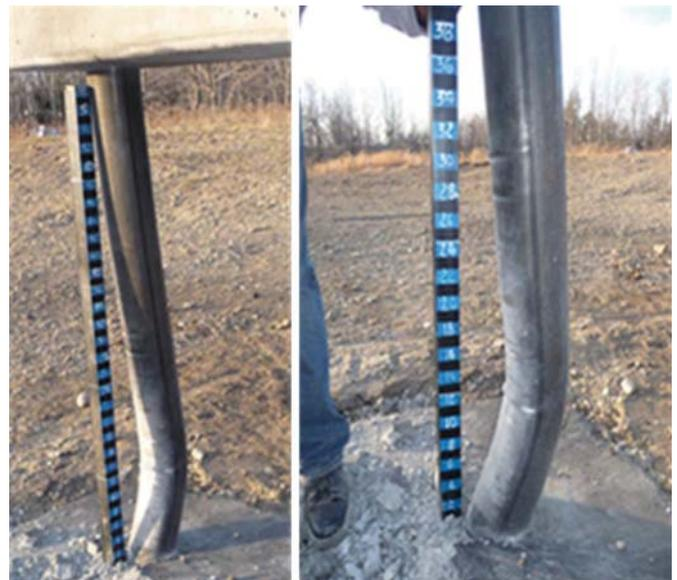
**Fig. 17.** View of the global deformation of Specimen B1
