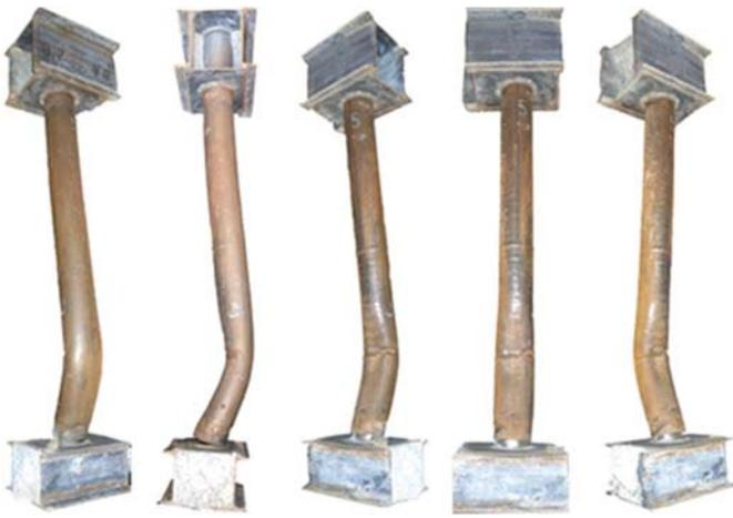
Fig. 18. Final deformed shape of Specimen B2
